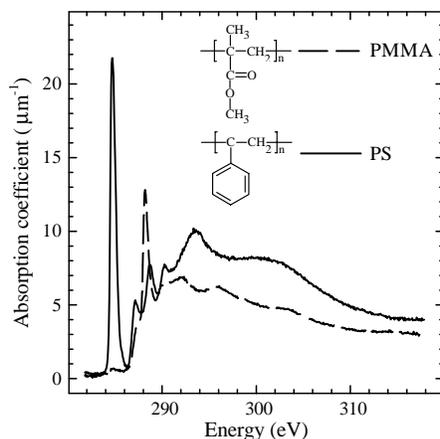
Fig. 1. – Reference spectra of PS and PMMA normalized to the pre- and post-edge linear absorption coefficients of Henke [11], assuming a density of  $1.07 \text{ g/cm}^3$  for PS and  $1.19 \text{ g/cm}^3$  for PMMA [12].
