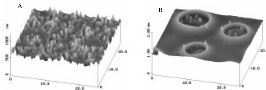
Fig. 4. – AFM topographs of samples with the surface PS removed with cyclohexane: after 10 min (A), and 64 h (B) of annealing.
