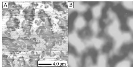
Fig. 3. – A Lateral force modulation and B topography maps of a sample annealed for 10 min.
