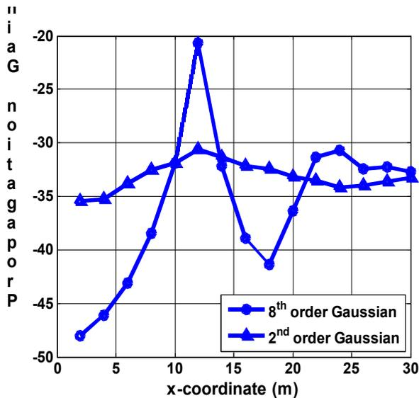
Figure 8. Comparison of propagation gain for the Gaussian monocycle pulses in Fig. 1 as the receiver moves along line A in Fig 5.
