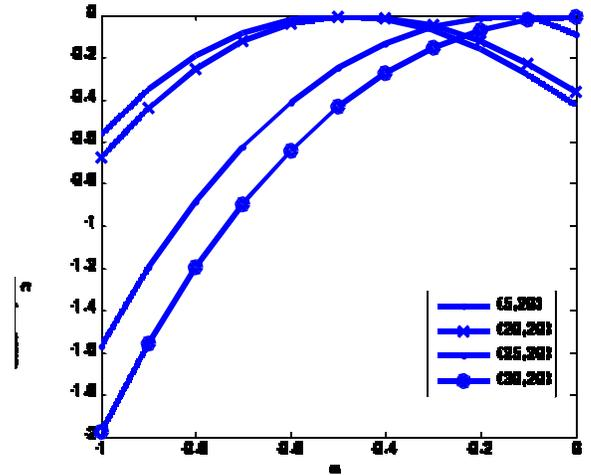
Figure 4. SNR<sub>c</sub> capture for fractional integral templates of order  $\alpha$  for receiver positions along line A in Fig. 2 (diffraction to LOS), 2<sup>nd</sup> Gaussian monocycle  $t_p=0.25$ ns transmit pulse.
