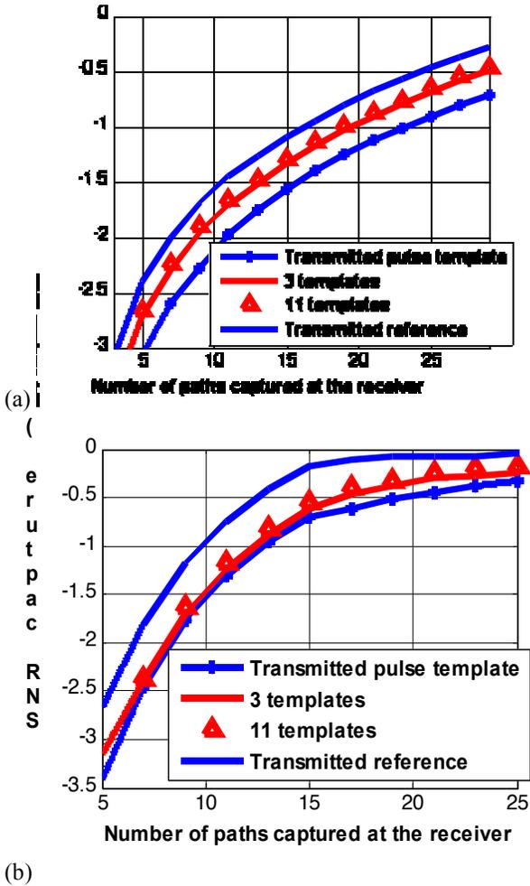
Figure 7. SNR capture as a function of the number of paths captured at the receiver position (3,15). Diffraction is the dominant propagation mechanism; 2<sup>nd</sup> order Gaussian monocycle transmit pulses: a)  $t_p=0.25\text{ns}$  b)  $t_p=2.5\text{ns}$
