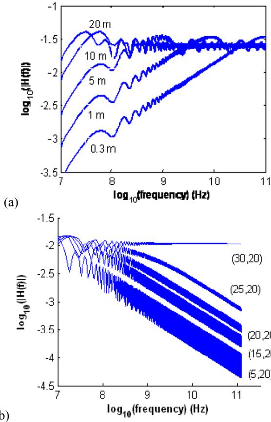
Figure 3. Amplitudes of frequency responses for paths in Fig. 2. (a) Path 3, reflectors of various sizes, receiver position at (10, 20) (b) Diffraction path for receiver positions along line A.
