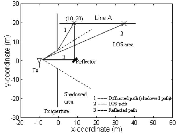
Figure 2. A simple geometry for the UWB physical model.
