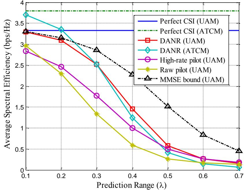
Fig. 3. Spectral efficiency vs. prediction range for SNR=20dB, Jakes model, and  $P_f=10^{-4}$
