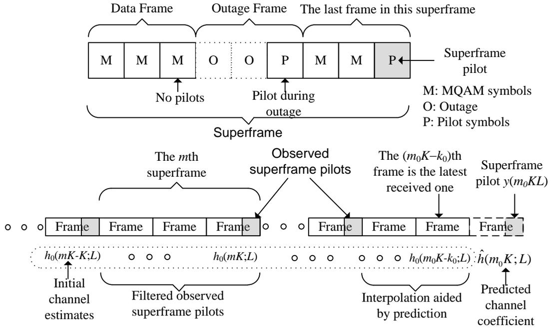
Fig. 1. Frame structure and initial channel estimates for demodulation (see equation (7)).  $L=3$  symbols/frame,  $K=3$  frames/superframe. (Keep this figure. Delete Fig. 1 and 2?)
