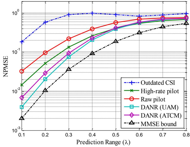
Fig. 2. NPMSE vs. prediction range for SNR=20dB, Jakes model, and  $P_f=10^{-4}$ . (UAM: uncoded adaptive modulation, ATCM: adaptive trellis coded modulation)
