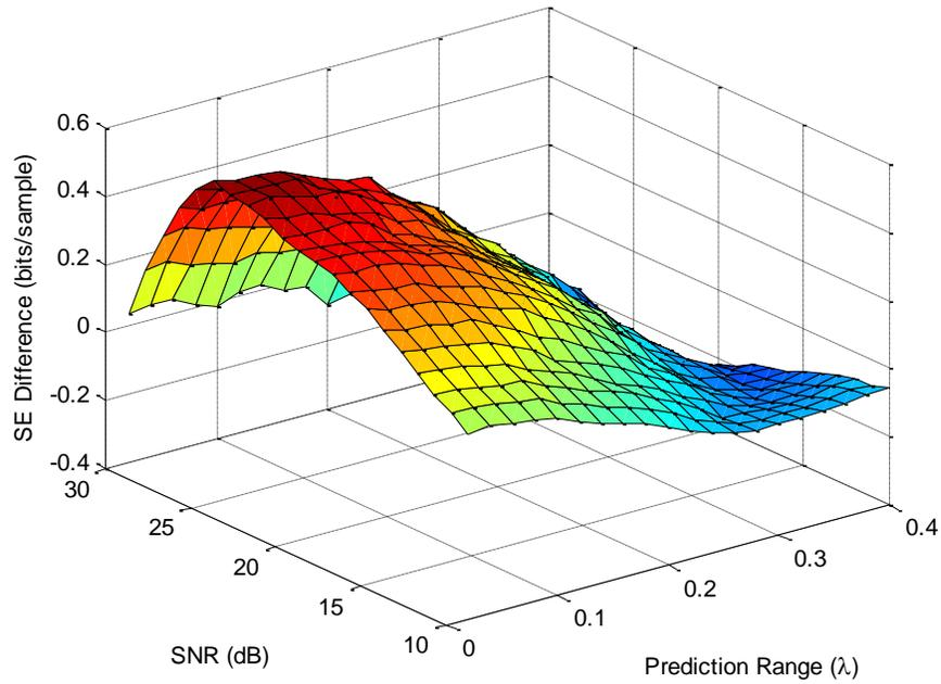
Fig. 6 (New Fig. 6) Difference in spectral efficiency between ATCM and uncoded adaptive modulation with LRP enabled by DANR for Jakes model and  $P_t = 10^{-4}$
