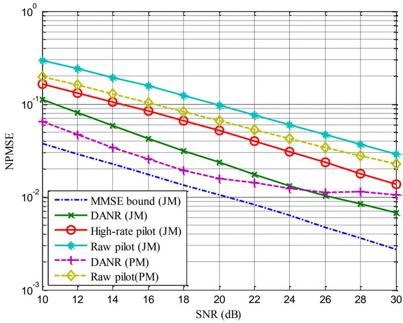
Fig. 4. NPMSE vs. SNR for prediction range at  $0.2\lambda$ , UAM,  $P_t=10^{-4}$ , Jakes model (JM) and physical model (PM) (New Fig. 4)
