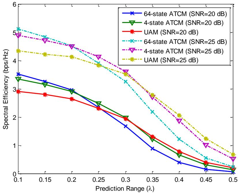
Fig. 7 Spectral efficiency vs. prediction range for Jakes model and  $P_t = 10^{-5}$  (UAM: uncoded adaptive modulation, ATCM: adaptive trellis coded modulation)
