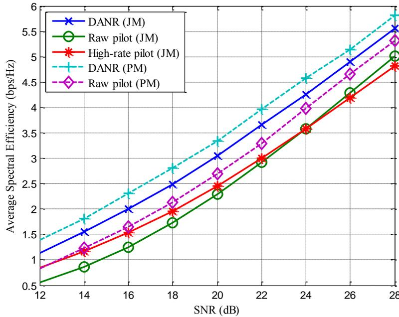
Fig. 5. Spectral efficiency vs. SNR for prediction range at  $0.2\lambda$ , uncoded adaptive modulation,  $P_t=10^{-4}$ , Jakes model (JM) and physical model (PM) (\*They are all about UAM\*)
