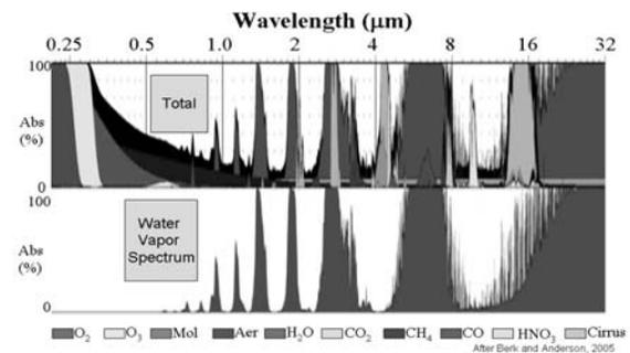
Figure 2. The optical transmission of the atmosphere between ground and space from MODTRAN<sup>5</sup> [2].
