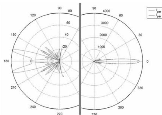
Figure 8. Scattering intensity distributions expected for 1  $\mu\text{m}$  particles scattering 0.5  $\mu\text{m}$  polarized light in directions parallel and perpendicular to the polarization plane (note the change in scale).
