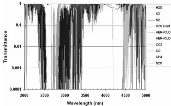
Figure 6. The optical transmittance of the MWIR between ground and space shows absorption lines for use in calculating species densities.
