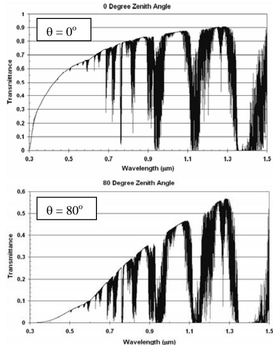
Figure 5. The atmospheric optical transmission between ground and space is shown from a MODTRAN<sup>TM</sup>4 model calculation for atmospheric paths at 0° and 80° zenith angles.
