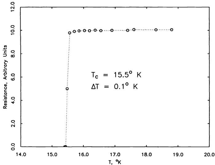
Figure 4. Resistance vs. temperature for a typical NbN film.
