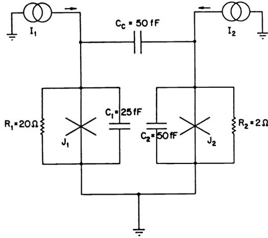
Figure 2. Equivalent circuit schematic for the double tunnel junction device.
